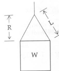
Double tension calculations if rope goes around sharp corners.
