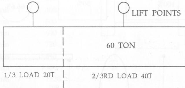
It is also possible to use an additional lifting beam to proportion lifts. Examples given are a two crane lift and a three crane lift.
