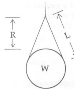
T x 1 1/2 for circular loads more than 10 times the diameter of the wire.
