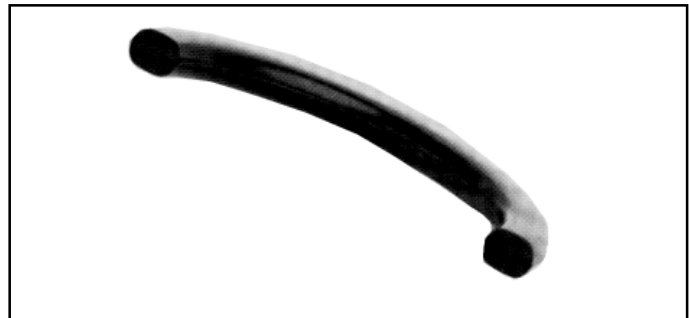
Figure 10-1: Characteristic compression set — high deformation
