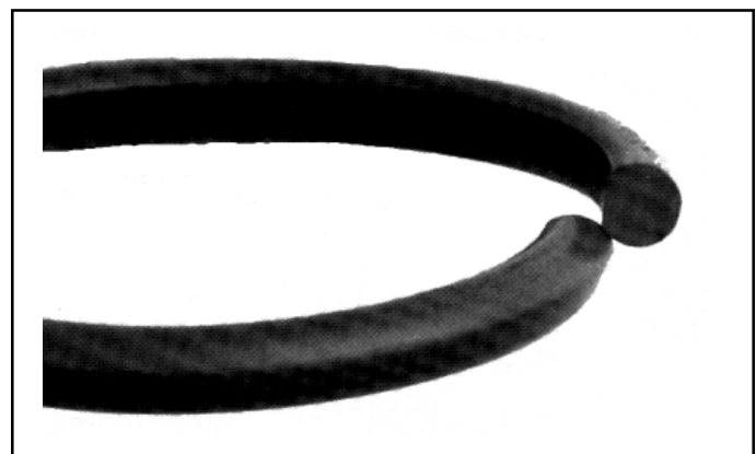
Figure 10-6: Wear is Seen as Flattening of O-ring on One Side
