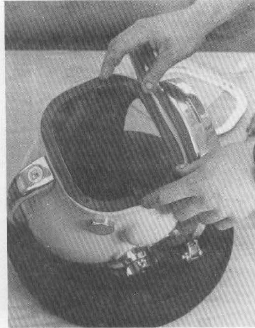
2. Thin coat of silastic on helmet side of gasket and place on port opening.
