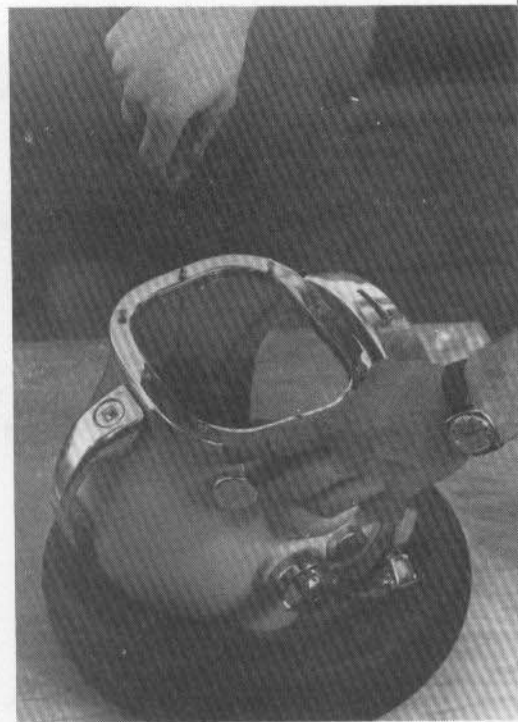
4. Insert and tighten bolts with Allen wrench. Clean off excess silastic with a clean rag and alcohol. Tighten evenly as you would the head bolts on an engine.
