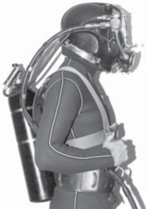
Diver with emergency gas supply connected to the helmet.
