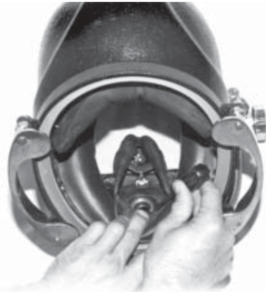
Pop the Oral Nasal tube into Fitting Groove with a blunt screwdriver.
