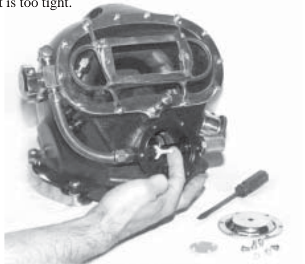
Check Free Movement and position of Lever (88).
