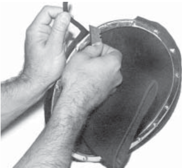
Trim excess rubber after installing new Neck Seal (18).
