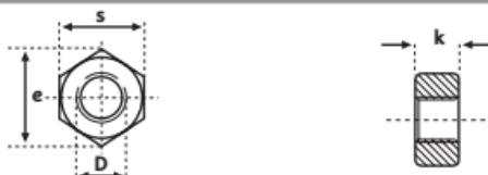
Metric threads, dimensions [mm] [DIN934]
