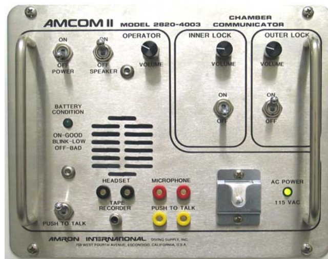
Figure 2-9. Control Console Communications Panel
