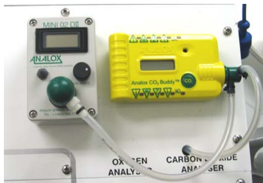
Figure 2-12. Air Sample Monitors
