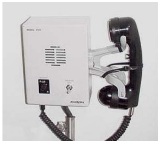
Figure 2-10. Interior Communications Panel
